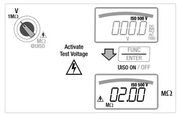
Auto-ranging is active during insulation resistance measurement.
